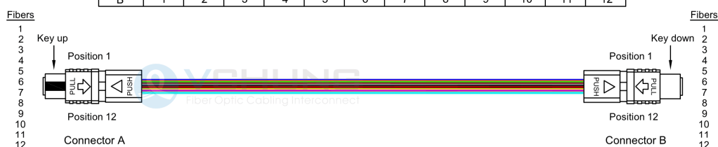
Type-B array patch cord fiber sequence
